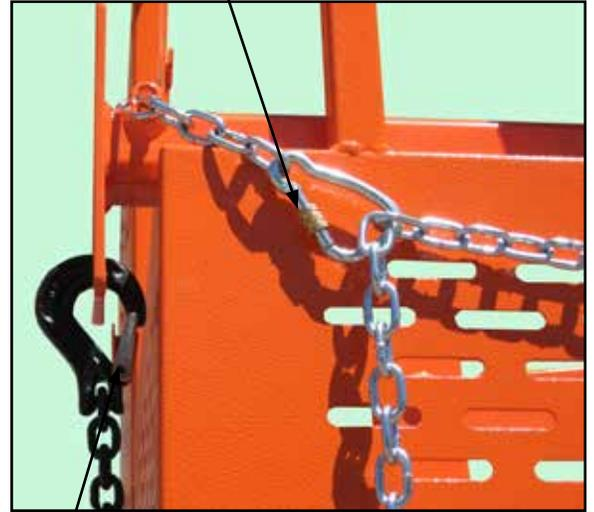
**Hook with safety latch to secure test weights to cross beams**
