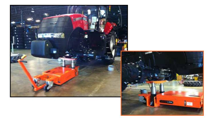
High capacity lifting device rated for up to 22.5 tons for mounting tires on tractors.
