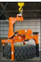
The SideWinder has the ability to lift tires from a horizontal surface, such as a pallet, rotate them to vertical and then install the tire onto the axle. This below the hook design combines the functions of a tilt table and tire handler into one compact piece of equipment that has a minimal footprint.
