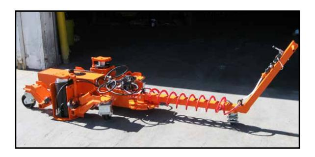
High capacity lifting device rated for up to 66 tons for mounting tires on articulated trucks.
