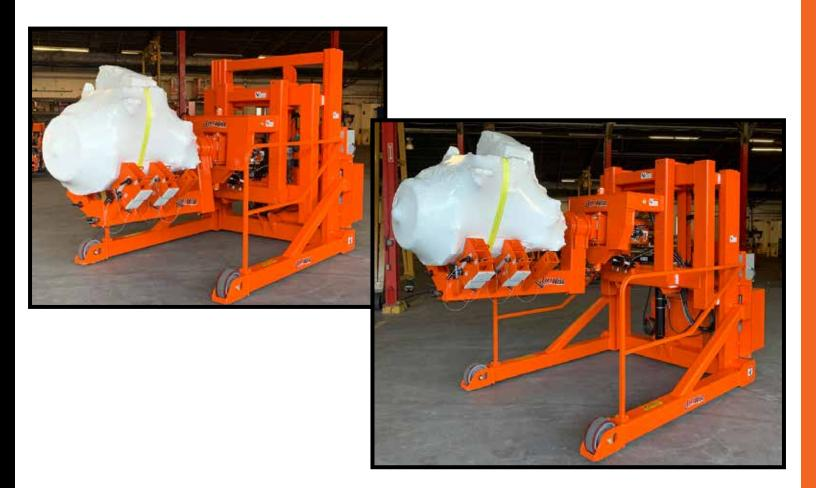
The Transmission Manipulator is a high capacity piece of equipment for handling, controlling and maneuvering transmissions on Wheel-Tractor Scrapers for installation, removal or maintenance. A transmission can be safely handled and precisely positioned by one person.
