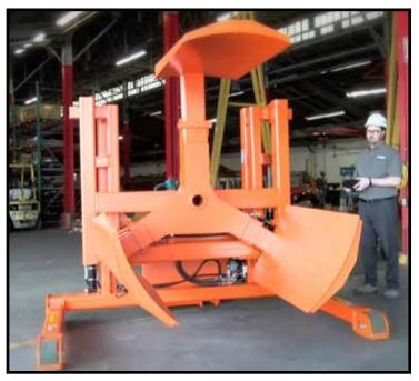
The Lift Wise 6500 Series Wheel Handler can mount tires ranging in size from 55" up to 79" in diameter and weighing up to 6,500 pounds. The wheel can be safely transported using the maneuverability and familiar controls of a pallet truck. The wheel then can be precisely positioned onto the truck by one person using the lift, side-shift, upper jaw, lower jaw and rotation functions on the hand-held, tethered controller.
