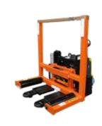
The LiftWise 3500 Series Tire Handler can mount tires ranging in size from 48" up to 86" in diameter and weighing up to 3,500 pounds. Various models are available that accommodate tire widths up to 32". The tire can be safely transported using the maneuverability and familiar controls of a pallet truck. The tire then can be precisely positioned onto the truck by one person using the lift, side-shift and rotation functions on the hand-held, tethered controller.
