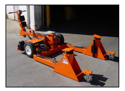
High capacity lifting device rated for up to 25 tons for mounting tires on articulated trucks.
