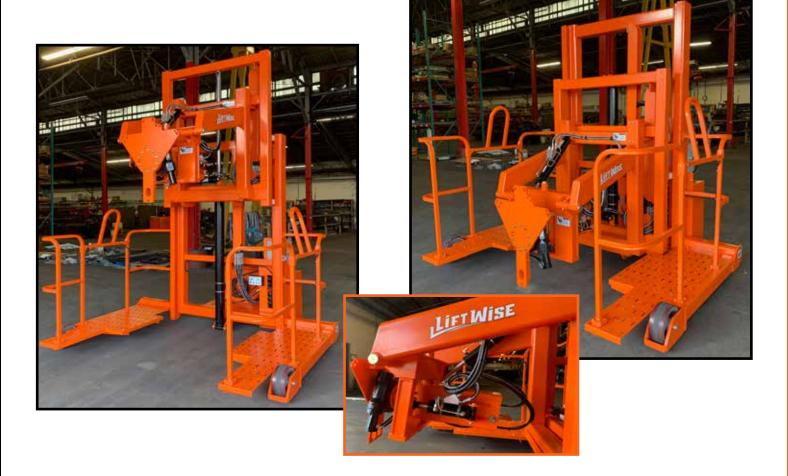
The Differential Manipulator is a high capacity piece of equipment for handling, controlling and maneuvering differentials of Wheel Tractor Scrapers for installation, removal or maintenance. A differential can be safely handled and precisely positioned by one person. The Differential Manipulator is also easily adapted to installing other components of similar size and weight.
