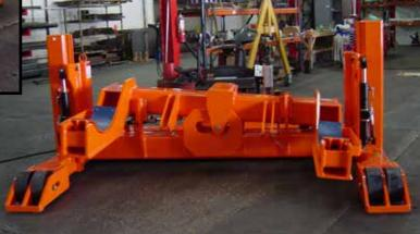
Mobile, self-powered device that installs rear axles on 40 ton to 70 ton mining trucks. 5 degrees of freedom for aligning the axle with the chassis and connecting the dogbone and struts.
