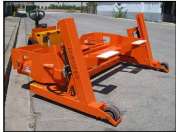
Custom handling device for installing A-frames (part that connects rear axle to chassis) on 40-ton to 240-ton rigid-frame mining trucks.
