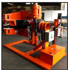
The LiftWise Rollover Stand is a piece of equipment for flipping cast iron and steel parts with circular outer surfaces ranging from 12" to 48" in diameter, 2" to 15" in height and up to 920lbs.
